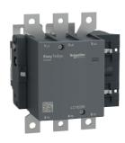
Contactor, Easy TeSys Control, LC1E, 3P(3NO), AC-3, <= 440V, 250A, 220V AC coil, 50Hz
